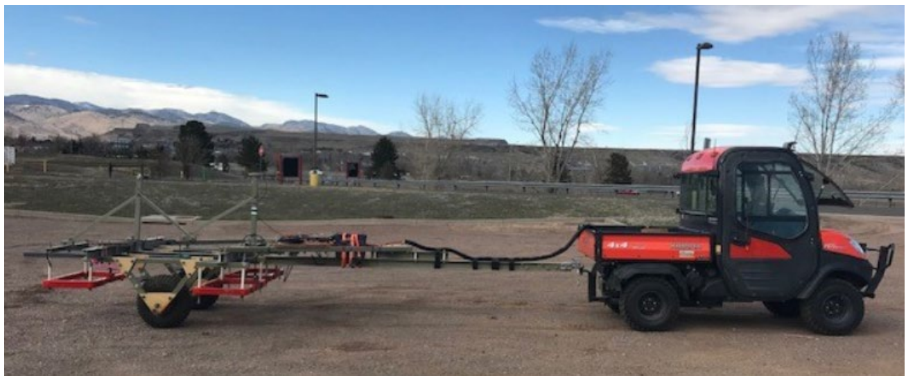
Figure 2-3. Photo of VTA 3-sensor Array and Tow Vehicle
